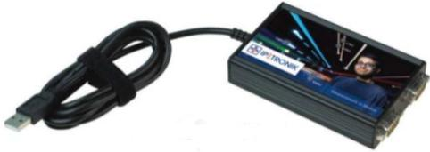
A rectangular CAN card with a blue and black label. It has a USB connector on one side and a DB9 connector on the other. A black cable is attached to the DB9 connector.           | <ul style="list-style-type: none"><li>• 输入: 2*高速 CAN ISO 11898-2 至 1MBit/s<br/>2*LIN 2.1 1kBit/s~20kBit/s</li><li>• PC 接口: USB2.0</li><li>• CAN 接口: DB9 公头, 针脚定义为 CIA<sup>®</sup>102 标准</li><li>• 通过 IPEmotion 进行配置和采集</li><li>• 供电: 5VDC(USB) 9~36VDC(DB9)</li><li>• 工作温度: -40~85°C</li><li>• 湿度: 15%~90%</li></ul> |
