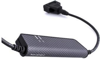
A rectangular CAN card with a black and grey label. It has a USB connector on one side and a DB9 connector on the other. A black cable is attached to the DB9 connector. | <ul style="list-style-type: none"><li>• 输入: 高速 CAN ISO 11898-2/</li><li>• PC 接口: USB2.0</li><li>• CAN 接口: DB9 公头, 针脚定义为 CIA<sup>®</sup>102 标准</li><li>• 通过 IPEmotion 进行配置和采集</li><li>• 供电: 5VDC(USB) 9~36VDC(DB9)</li><li>• 工作温度: -20~75°C</li><li>• 湿度: 15%~90%</li><li>• 光电隔离</li></ul>                            |
