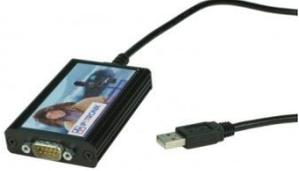
A small, rectangular CAN card with a blue and black label. It has a USB connector on one side and a DB9 connector on the other. A black cable is attached to the DB9 connector.         | <ul style="list-style-type: none"><li>• 输入: 高速 CAN ISO 11898-2/</li><li>• PC 接口: USB2.0</li><li>• CAN 接口: DB9 公头, 针脚定义为 CIA<sup>®</sup>102 标准</li><li>• 通过 IPEmotion 进行配置和采集</li><li>• 供电: 5VDC(USB) 9~36VDC(DB9)</li><li>• 工作温度: -40~85°C</li><li>• 湿度: 15%~90%</li></ul>                                           |
