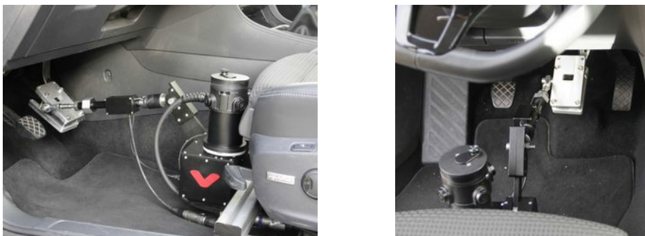
Illustration 13: Pedal Robot CP800
