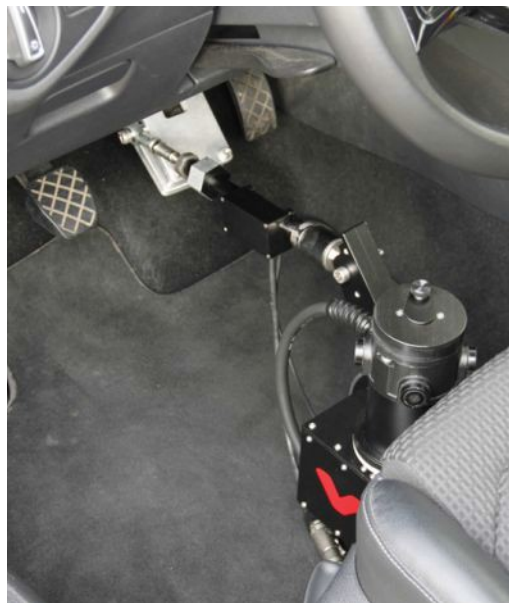
Illustration 12: Installation of Pedal Robot CP800 between Seat and Pedal
