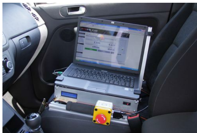
Illustration 15: The VEHICO Robot Controller installed on the Passenger Seat
